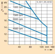
Minimum cantilever force 5 kN  $L_{10h} = 12000 h$
