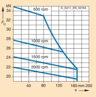
Minimum cantilever force 9 kN  $L_{10h}$  >12000 h when regreased
